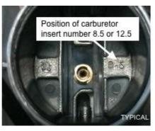
Angular bore: Plug gauge 0.60 may not fit. (8.5 Carburettor Insert only) (Use jet gauge set ROTAX part no. 281 920)
