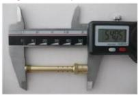
17.14.2 Length of bottom section of needle jet: 11.50 +/- 0.2mm
