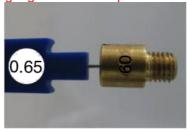
17.16.2 Plug gauge 0.65mm may NOT enter the bore of the idle jet insert 60 (Use jet gauge set ROTAX part no. 281 920.
