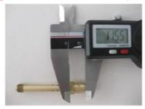
17.14.3 Top bore diameter of needle jet 2.60 +/- 0.15mm
