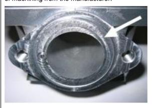
5.7.4 The top edge of the exhaust port may show either just a cast finish surface...
