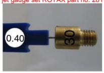
Plug gauge 0.40mm may NOT enter the bore of the idle jet insert 30 (Use jet gauge set ROTAX part no. 281 920.
