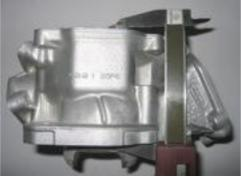
5.7.1 All transfer ports and passages have cast finish surface except some removal (done by the manufacturer) of cast burr at the inlet passage. and exhaust port and passages. All ports have chamfered edges to prevent ring snagging. Any additional machining is not permitted. The top edge of exhaust port may show some preexisting machining from the manufacturer. The sealing flange for the exhaust socket may show signs of machining from the manufacture.
