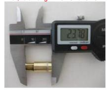
17.18.2 Atomizer, length of cylindrical part: 15.75 +/- 0.25mm
