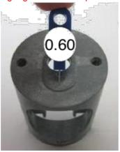
Vertical bore: Plug gauge 0.90 may not fit. (8.5 Carburettor Insert only) (Use jet gauge set ROTAX part no. 281 920)
