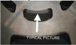
5.7.3 The sealing flange for the exhaust socket may show either cast finish surface or signs of machining from the manufacturer.
