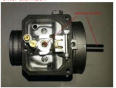
17.18.1 Remove atomizer from carburettor body using venturi tool set (ROTAX part no. 676034): Atomizer, total length: 23.75 +/- 0.45mm
