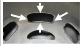
On cylinders marked 613 993 the upper edge of the central boost port may show factory machining.
