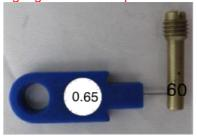
17.17 Carburettor insert must show number stamping of either 8.5 or 12.5 as illustrated below.
