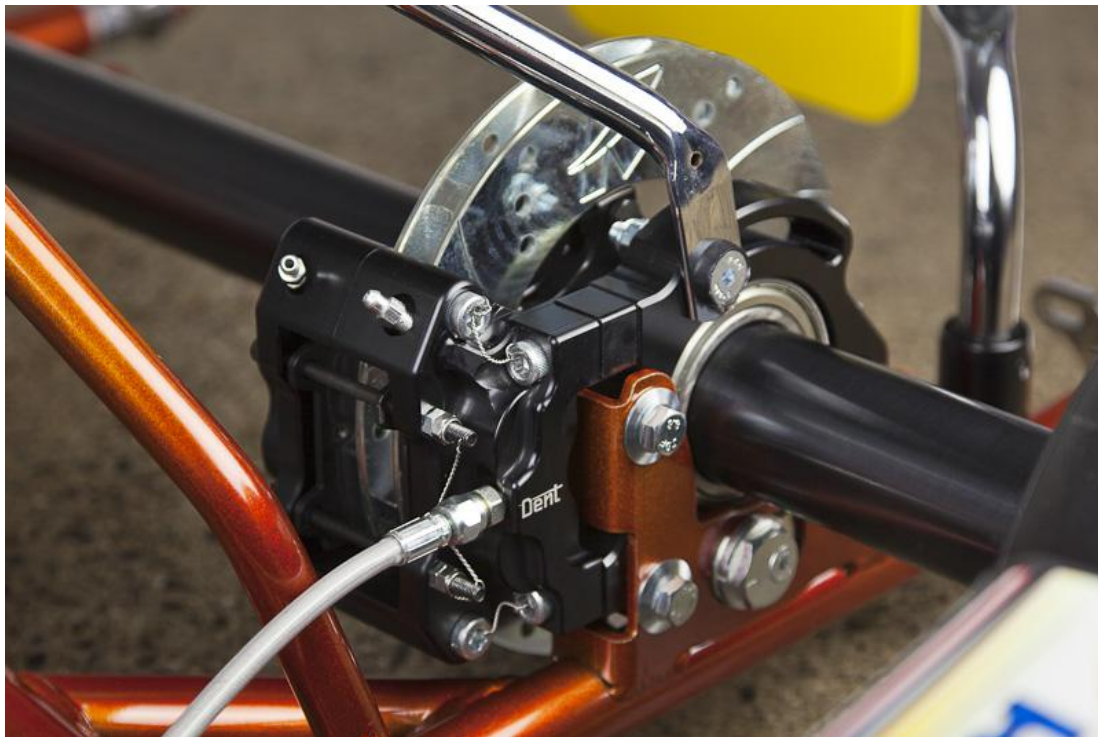
Self-Adjusting brakes, standard on CIK, KZ, DD2, & Cadet/Rookie. Optional on 28C
