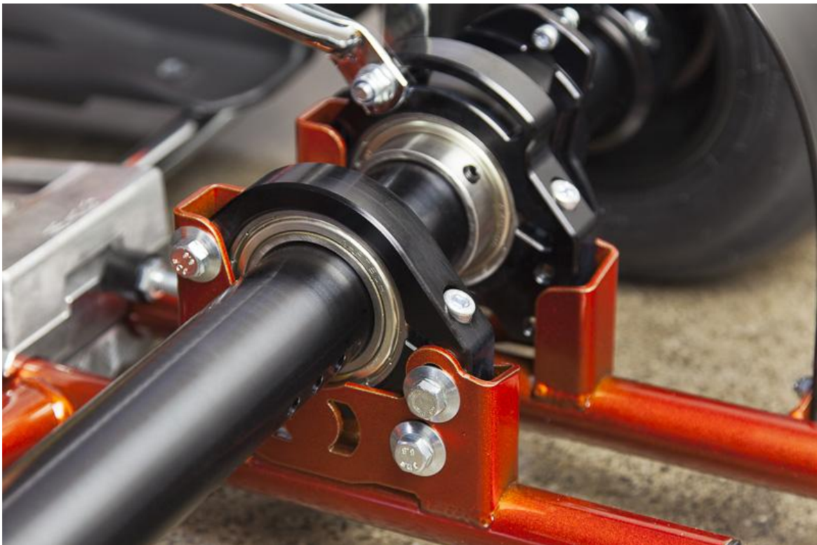
Monaco's new seat stay / ride height adjustable bearing flanges, eliminates the need for additional length seat stays
